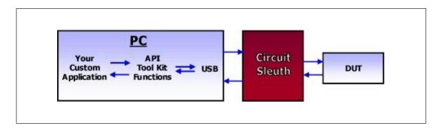
The architecture of the interface consists of USB drivers (installed with the Circuit Sleuth application installation disk) that communicate with the analyzer hardware, and a set of function calls from the API Tool Kit.
